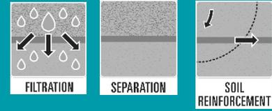
Mirafi® HP270 geotextile is composed of high-tenacity polypropylene yarns, which are woven into a network such that the yarns retain their relative position. Mirafi® HP270 geotextile is inert to biological degradation and resistant to naturally encountered chemicals, alkalis, and acids.
